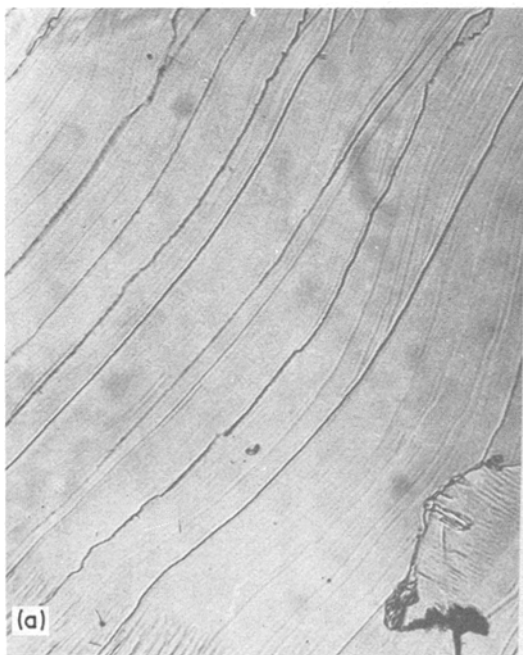
Figure 2 (a) A typical (110) cleft plane exhibiting smooth cleavage lines ( \times 180 ). (b) A multiple beam interferogram over the region of the face shown in (a) revealing the perfect nature of the crystal cleavages ( \times 180 ).
